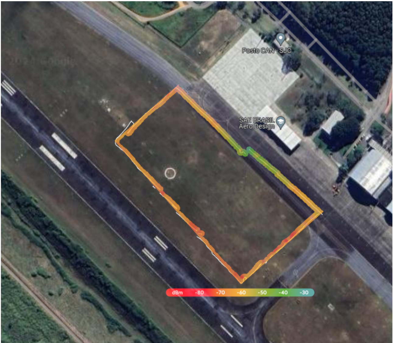
Figura 12.9: RSSI Measurement for AP01
