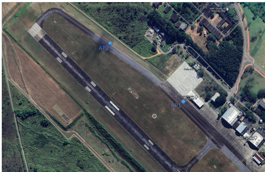
Figura 12.2: Transceivers positioning in satellite view
